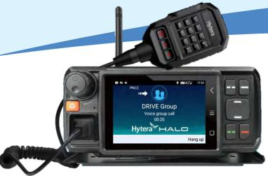
The MNC580 and other Hytera PoC devices are part of the Hytera HALO Nationwide PoC solution that uses cellular 3G/4G/LTE infrastructure, the Hytera HALO Connect unified PoC and LMR platform, and third-party Push-to-Talk over Cellular plans. The MNC580 is supported on Hytera HALO Dispatch, a powerful web-based GPS dispatch and fleet communications application.
