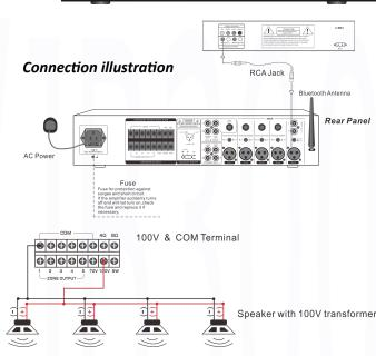
The JB150/JB300 5 Zone PA Installation Amplifiers are designed with a 2U height housing including removable rack mounting brackets, and overall 4/8 ohms( $\Omega$ ) loads and features an industry leading 5 zoned 100 volt and 70 volt load solution.
