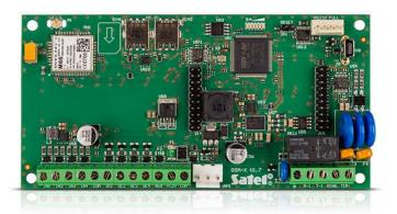
As for the INTEGRA and INTEGRA Plus control panels, connection with them can be via RS-232. Thus, GSM-X will perform reporting and notification (in INTEGRA Plus), the content is downloaded from the list of events), and will establish remote connection with DLOADX and GUARDX programs.
